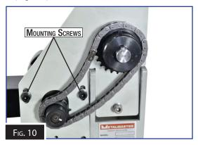
11. Once the chain has been tensioned, using a straight edge adjust the sprockets so that they are aligned and the chain drive will operate correctly. Once this is done " then tighten the grub screws on the sprockets. (Fig. 11)
