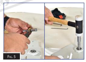
6. Secure the idler shaft with the brass washer and then a circlip. Using the 4 socket head cap screws secure the motor to the new mounting plate (Fig. 6)
