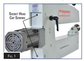
3. Remove the motor from the machine. (Fig. 2)
